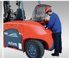
合适的电控仓高度、锁定型牵引销 Comfortable height of operation of electric control warehouse and lock-type traction pin
