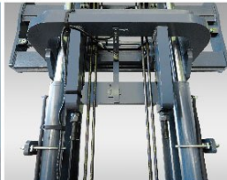
起升末端缓冲 Terminal buffer of lifting
