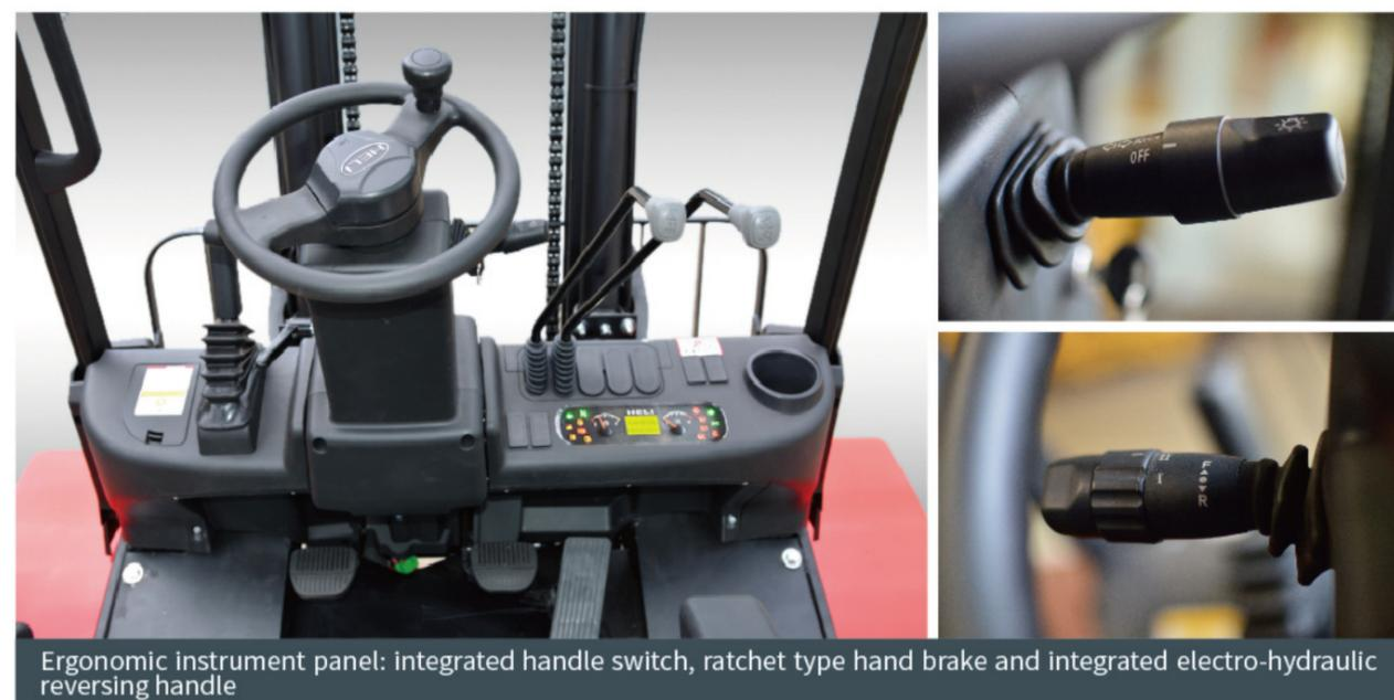
Ergonomic instrument panel: integrated handle switch, ratchet type hand brake and integrated electro-hydraulic reversing handle
